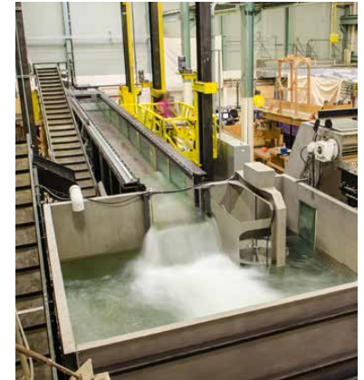
Above, top: Hima Hassenruck-Gudipati, a senior studying mechanical engineering, pours sediment into a feed system for Mike Lamb's delta experiments in the Earth Surface Dynamics Laboratory. Above, bottom: To better understand the damage flowing water can cause, Lamb built several different kinds of artificial waterways, called flumes. The tilting flume pictured can be slanted to a steep 18 degrees; Lamb and his team can then send up to 10,000 gallons of water per minute—enough to transport fist-sized rocks and other types of debris—down the incline. The setup allows the researchers to gain insights into the consequences of mountain flooding while also predicting the impact of water erosion and its role in the evolution of mountain ranges over geologic time.
