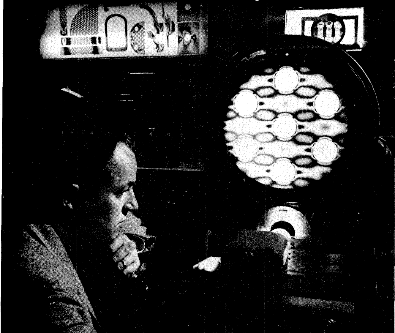
Westinghouse scientist Robert Sampson analyzes a special photoelastic model under polarized light to calculate the stresses which would be built up in an atomic reactor component now in the design stage.
