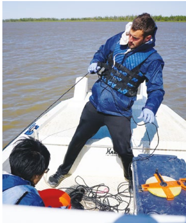
Caltech postdoctoral scholar Gerard Salter retrieves a water sampler from the Wax Lake Delta while Caltech graduate student Justin Nghiem (MS '21) readies the sample bag. Samples are analyzed for suspended mineral sediment and particulate carbon to predict land loss in the Mississippi Delta region as part of the JPL-led Delta-X project.
