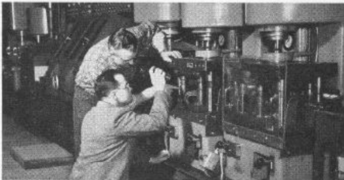
Here Dick and a set-up man check over the automatic production line used to manufacture a wire spring relay part for complex telephone switching equipment. This automatic line carries a component of the relay on a reciprocating conveyor through as many as nine different and very precise operations—such as percussive welding in which small block contacts of palladium are attached to the tips of wires to within a tolerance of \pm .002 ".
