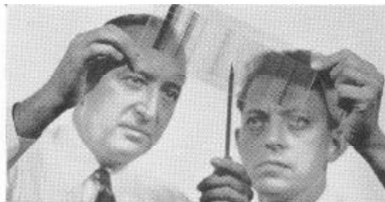
At Great Lakes Steel a spectrogram is readied for reading in the densitometer—one of the tests that assure quality steel.
