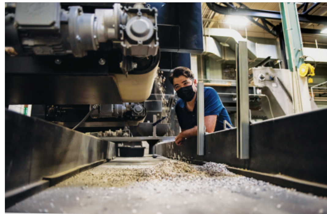
Professor of Geology Mike Lamb oversees work in the Caltech Earth Surface Dynamics Laboratory, where his team builds artificial rivers to simulate natural processes.
