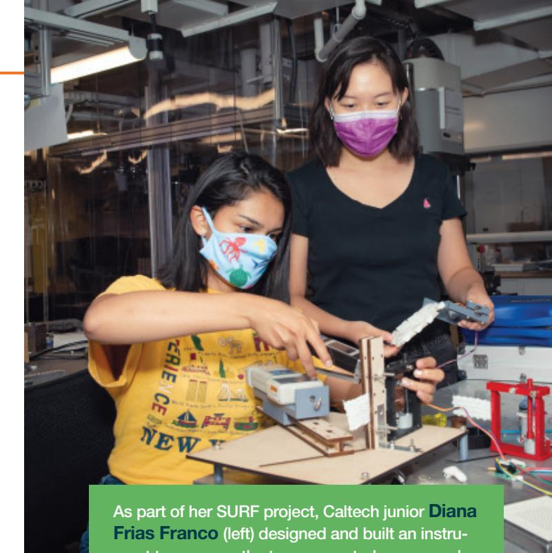
As part of her SURF project, Caltech junior **Diana Frias Franco** (left) designed and built an instrument to measure the torque exerted on a sample of smart fabric, an engineered wearable material that senses environmental stimuli and responds to varying conditions with changes in mechanical properties such as stiffness. She worked with **Chiara Daraio**, G. Bradford Jones Professor of Mechanical Engineering and Applied Physics.
