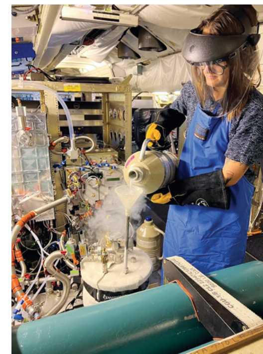
Graduate student Kat Ball fills a cryogenic pump with liquid nitrogen. The pump keeps her instruments clean during the downtime between flights.
