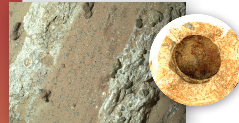
NASA’s Perseverance Mars rover used its Mastcam-Z instrument to capture this view of the Cheyava Falls rock sample within the rover’s drill bit.
