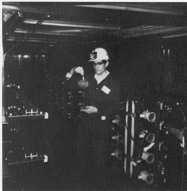
At left, the proton detector pit, 60' x 80' x 70' and 2000' underground, is lined with thick black plastic before being filled with water. Below, John LoSecco displays one of the 2048 photomultiplier tubes (others are lined up behind him) that will pick up the signals of decaying protons.
