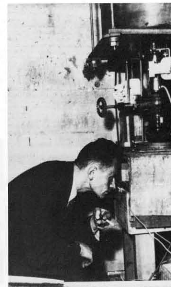
An ion beam tube (above) was built in the High Voltage Lab by C. C. Lauritsen and Dick Crane in 1932. What is now called the “experimental area” was located in the concrete block house beneath the tube. Count Soltan (below) is in this area peering at a Lauritsen electroscope next to the target, which is behind lead shielding.
