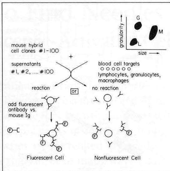
binding is detected by adding a fluorochrome-conjugated rabbit antibody against mouse or rat immunoglobulin (illustrated above). Because the sorter can measure additional properties of the target cells, it can discriminate between binding to the targets of interest and binding to some other cell type or to debris that may contaminate the target sample.
