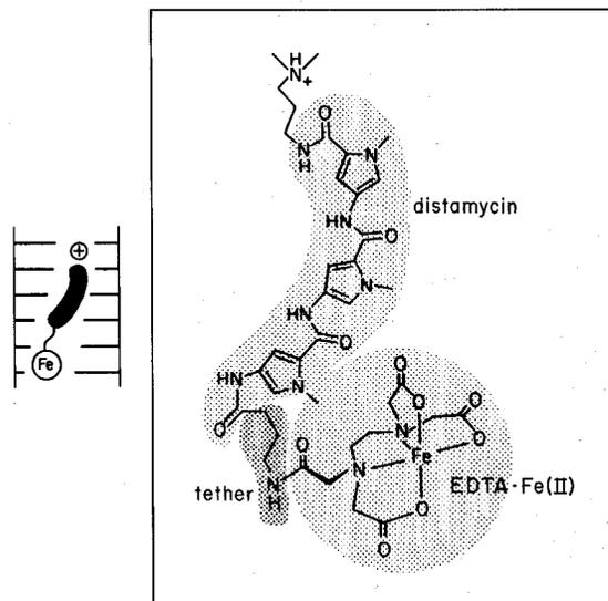
The banana-shaped antibiotic distamycin binds to DNA at a four-base-pair site by fitting into a groove of the double helix. By tethering the EDTA wrecking ball to the distamycin, the DNA can be cut at the specific site.
