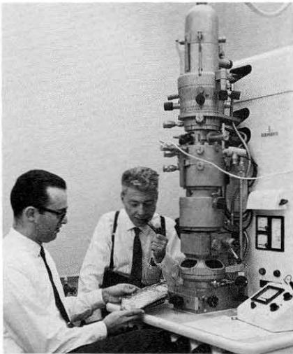
*In 1965 Duwez and Ronald Willens (BS '53, MS '54, PhD '61), assistant professor of materials science, were using an electron microscope to check the structure of alloys made with the rapid cooling technique.*
