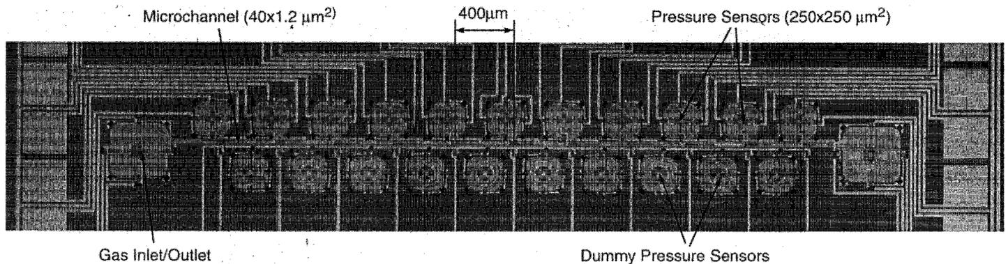
**Above: The uniform—flow micro wind tunnel. The channel is 4.5 millimeters long by 40 microns wide by 2 microns deep. The structure at one end is labeled “Gas Inlet/Outlet” because the tunnels are designed to accommodate flow in either direction. The “dummy” sensors along the bottom side of the tunnel provide for leak checks during the fabrication process.**
