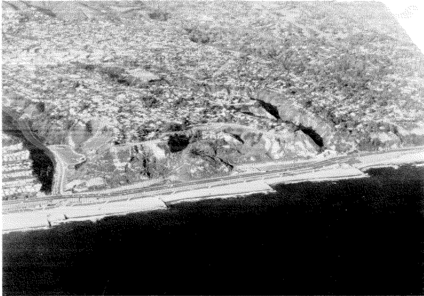
This series of groins (or jetties) that reach out into the ocean were placed along the beach at Pacific Palisades to stop the movement of sand, and they now provide a good illustration of how the natural transport of beach sand works. Wave action piles up sand on the north side of the groins, depleting the beach to the south. The effects of this interference would be much more severe at Santa Monica beach immediately to the south, if it were not for substantial artificial nourishment of that beach.
