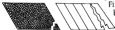
The polycrystalline diamond blank microfractures because of its structure. Natural cleavage planes of mined diamond (right) cause it to break off in larger pieces.
