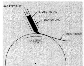
extremely well, and the formation of a melt puddle with the ribbon coming off is an extremely stable configuration. An iron-based alloy or steel can be continuously cast at the rate of a million degrees per second.
