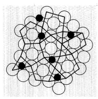
The holes in the liquid five-neighbor packing offer little extra spaces to put carbon or boron atoms (dark circles), forming an alloy, here  $Fe_{80} B_{20} - 80\%$  iron, 20% boron. This also stabilizes the configuration and makes it more competitive with the six-neighbor packing of the solid crystal.
