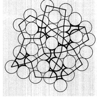
In a liquid metal, which has expanded, there will be many atoms that have only five neighbors. Conjoining five-sided figures doesn't work out as neatly as the hexagonal configuration; when you try to arrange the atoms in a regular periodic array, they fit together only by leaving holes, or defects — indicated here by the triangles between pentagons over the heavier lined spaces.
