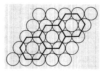
Seen in two dimensions, the atoms of this "perfect crystal" of iron arrange themselves most efficiently by lining up with six neighbor atoms, creating a neat hexagonal symmetry.
