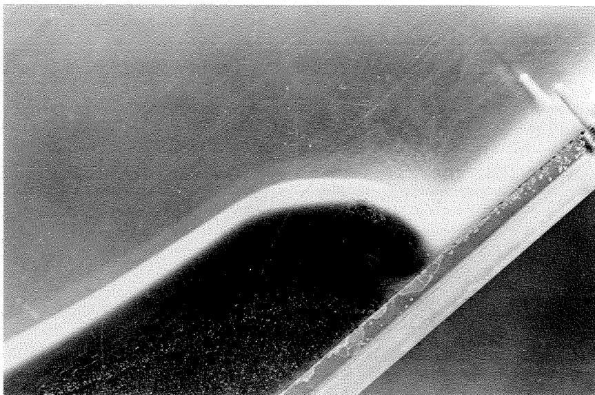
The backed up stationary layer of sand can be seen in this cross-sectional view of the "hydraulic jump" experiment. There is another very interesting spot of stationary granules near the top of the curve, where a vortex is created adjacent to the main flow. Lighting from above makes the top surface appear light.
