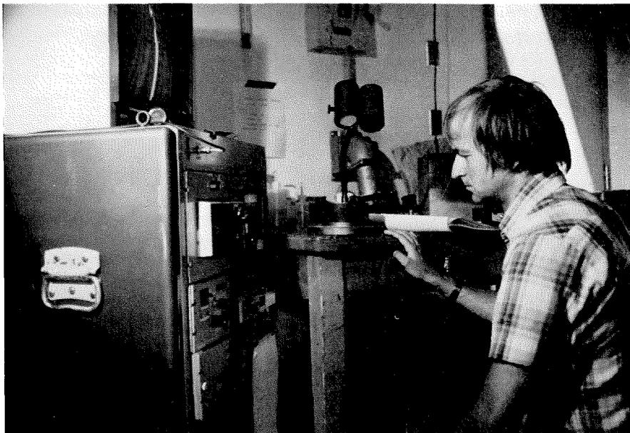
*To study dwarf galaxies, which are nearby and have easily detectable globular clusters, Jeremy Mould uses the data recording system of the CCD (charge-coupled device) camera at Palomar Observatory. The picture is displayed a few seconds after it has been taken.*
