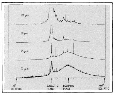
A scan across half the celestial sphere crossing both the galactic plane and the ecliptic plane of the solar system. produced these data from the four infrared telescope focal plane detectors, one for each of IRAS' wavelength bands. Cool dust from the galaxy produced peaks in the 60- and 100-micron regions (as well as some stars and hot dust in the 12- and 25-micron bands). Warm dust particles in the solar system radiate strongly at 12, 25, and 60 microns, but only weakly at 100 microns.
