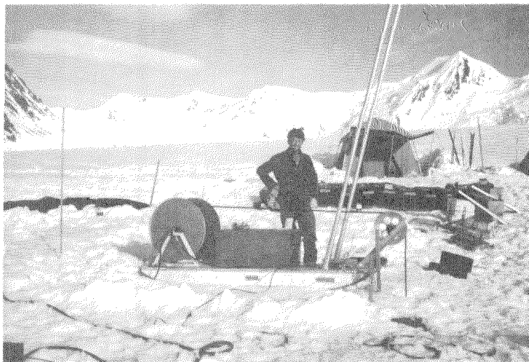
With jets of hot water, boreholes were drilled to the bottom of the glacier to measure its movement and the basal water pressure. Here Barclay Kamb poses amid the pieces of drilling equipment, which occasionally turned temperamental and got stuck in the ice.
