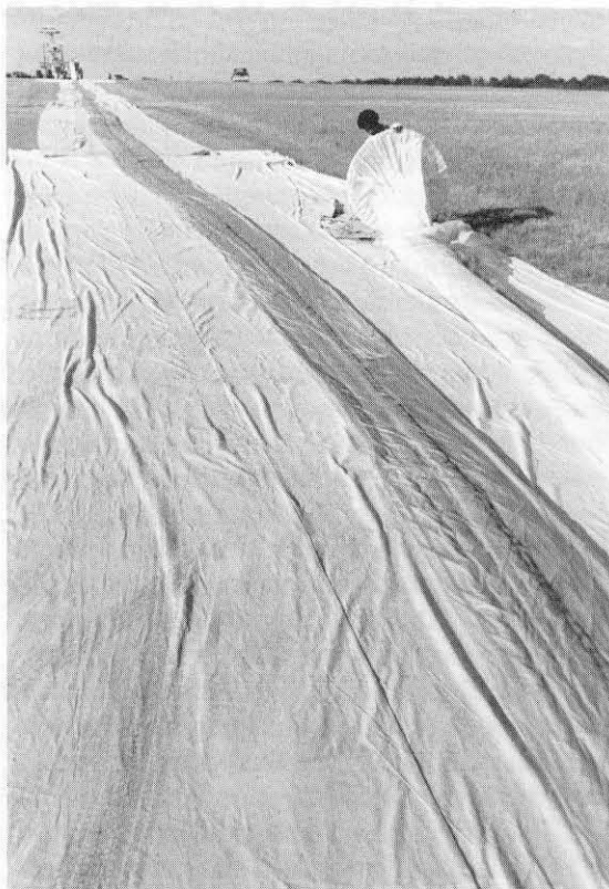
The unwieldy, giant balloon is hauled out of its crate and laid along the ground cloth (left); then the filling begins and the balloon swells into shape.
