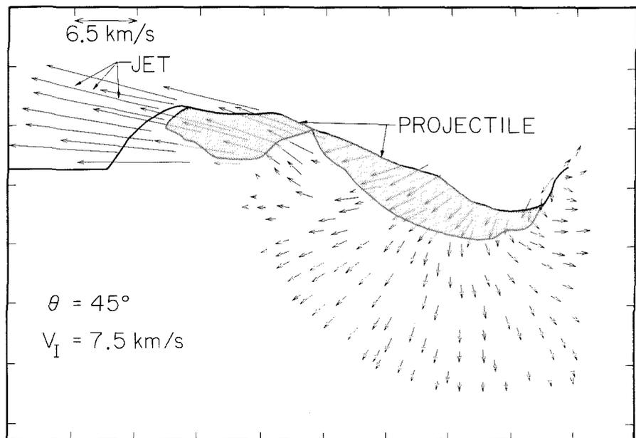
*In this simulated meteorite impact, a spherical object has just hit the Martian surface at 7.5 km/sec and at an angle of 45°. The impact produces a high-velocity jet of hot gas that can lift large boulders into interplanetary space. The arrows point in the direction of motion. Lengths are proportional to velocity.*
