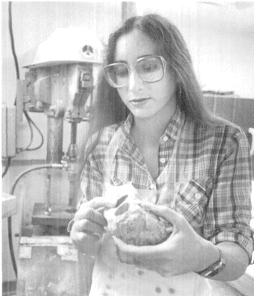
Janet Boley points to a core hole she drilled in one of the putative ancient hearth-stones. She'll slice the core itself like a salami and will measure the magnetic moments of the resulting discs.
