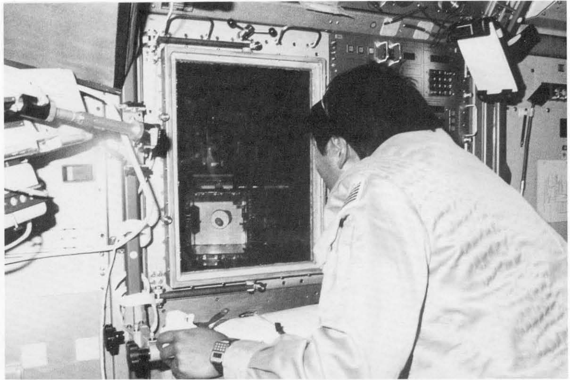
Right: Wang conducts an experiment involving a one-inch drop, visible in the chamber of the Drop Dynamics Module. The DDM uses sound to position and manipulate the drop without any physical contact. The image below is not actually a drop but a one-inch ball used for calibration of the instrument.
