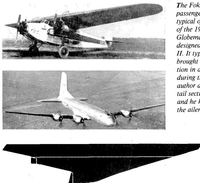
The Fokker Trimotor 10-passenger transport (top) was typical of the intuitive designs of the 1920s. The Douglas Globemaster (bottom) was designed during World War II. It typifies the changes brought about by the revolution in aeronautical science during the 30s and 40s. The author designed the wing and tail sections on this airplane, and he holds the patents on the ailerons and flaps.
