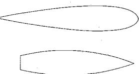
*Figure 2: The airfoil or airship (top) is the aerodynamicist's concept of a well-streamlined shape. In contrast, the typical boat shape (bottom) is designed to travel the other way around.*
