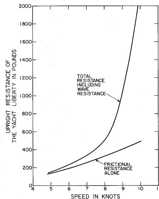
Figure 5 shows results from towing tank tests on a one-third-scale model of the 12-meter yacht Liberty. Note how wave formation causes the total resistance to rise rapidly at higher speeds.
