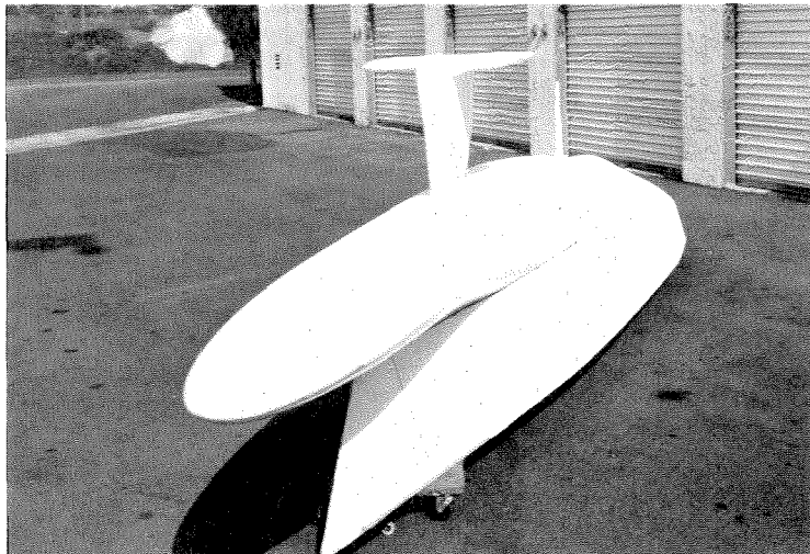
Figure 13 (above left): Since the power of the ailerons goes up with the square of the boat's speed, a yacht with ailerons could take full advantage of high winds. A conventional yacht would have to reef its sail, thus leveling off its speed, to keep from heeling too far.
