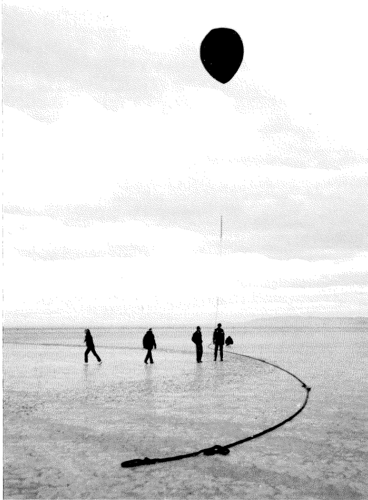
On the dry lake bed at Edwards Air Force Base a team from JPL and Caltech conducts a flight test of a Montgolfiere balloon with a segmented payload and drag rope, which might be used to keep a balloon's height constant above the Martian terrain.
