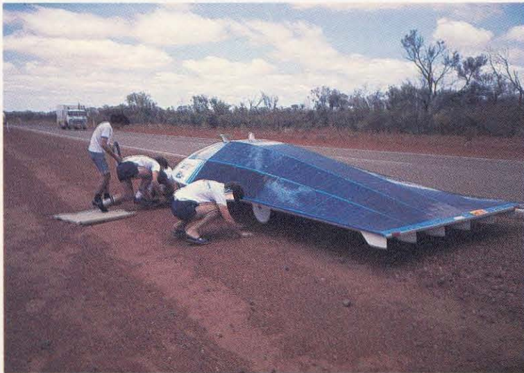
The crew changes one of three flat tires during the race. Stopping, changing the wheel, and reaccelerating took only about two minutes.
