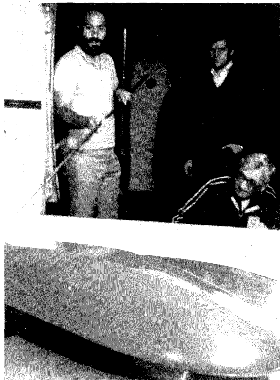
This quarter-scale model of Sunraycer scored the lowest drag coefficient ever recorded for a land vehicle in Caltech's 10-foot wind tunnel. From left to right Bart Hibbs, Max Schenkel, and Kent Kelly view the tests.
