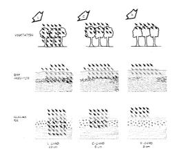
Microwave radars penetrate to different depths, depending on the wavelength.
