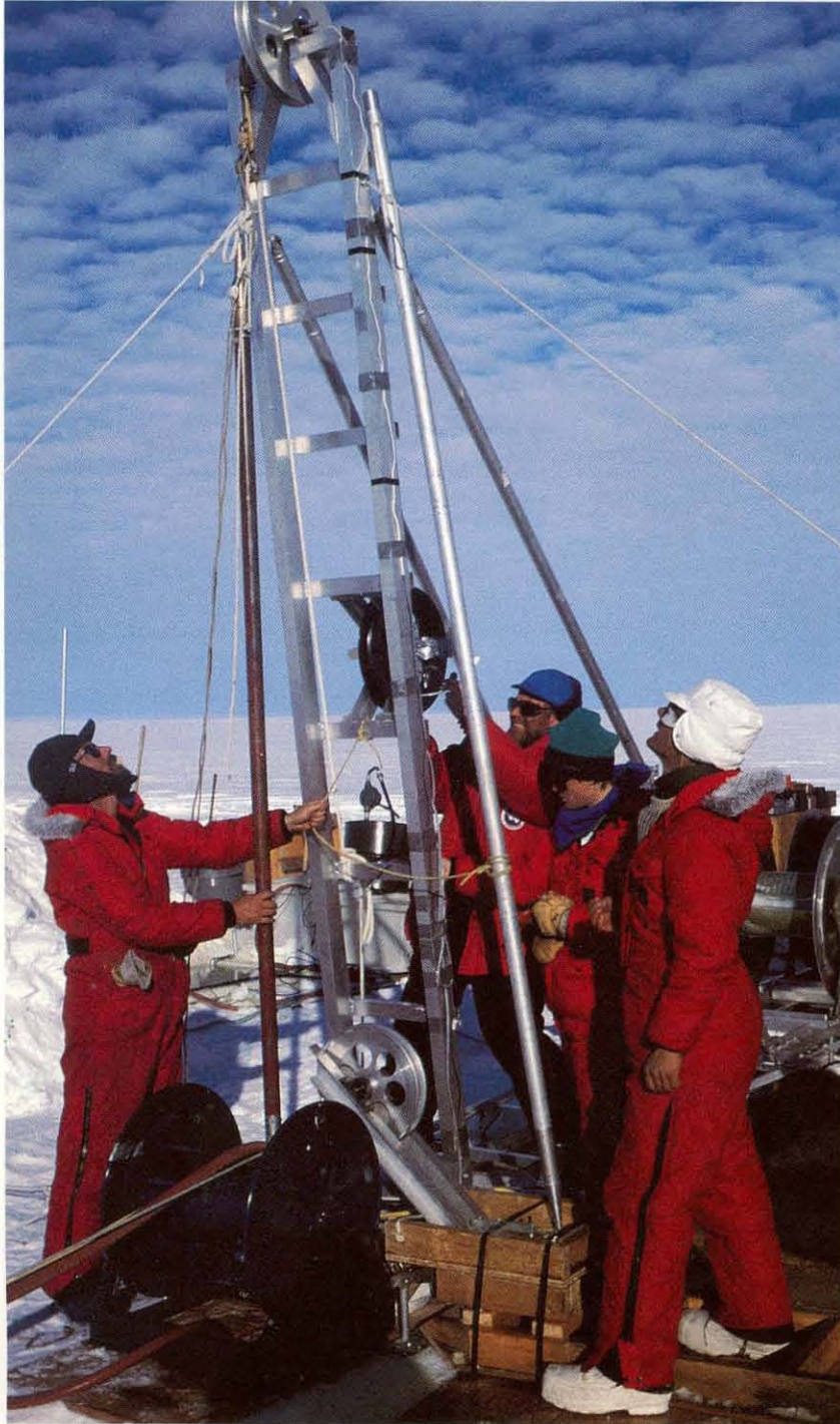
Preparing to lower a core drill to the base of the ice stream are (from left) Howard Conway, Hermann Engelhardt, Judy Zachariasen, and Neil Humphrey.
