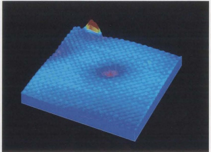
**Top right:** STM reveals the surface atomic lattice of gallium arsenide. The 125-angstrom-square image, made by grad student Robert Driscoll, resolves the gallium atoms along with an adsorbed electro-negative defect (magenta depression in center). The height of the atomic corrugation is 0.03 angstroms.
