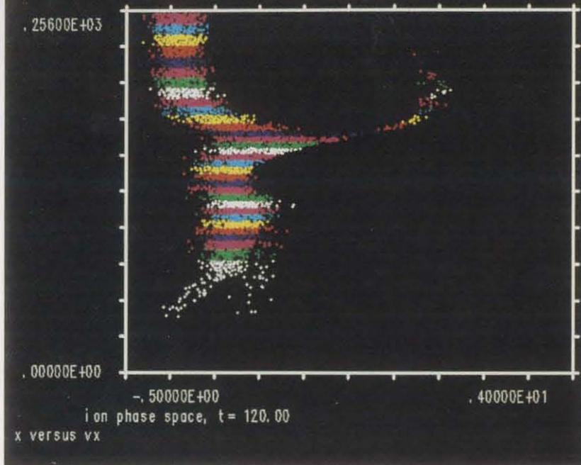
**A simulation of the earth's bowshock shows the solar-wind ions streaming in from the top and slowing down as they hit the shock about a third of the way down. The vertical axis represents ion position, and the horizontal axis, velocity. Each color stands for ions in the region of space tracked by one processor of the Mark IIIfp.**
