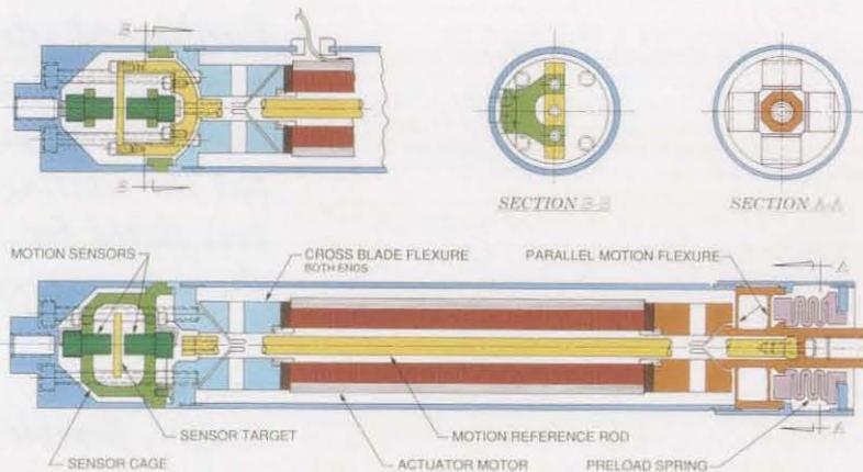
**The piston's innards (above). Like a chainsaw-cut tree that's ready to topple, the "cross blade flexure" (upper right) is almost sliced through, tapering down to two thin, flexible regions—the "blades"—at right angles to each other. The blades absorb any sideways load on the piston. The "preload spring" (lower right) is really four springs in one. The machining was done in the Lab's own high-tech machine shop.**
