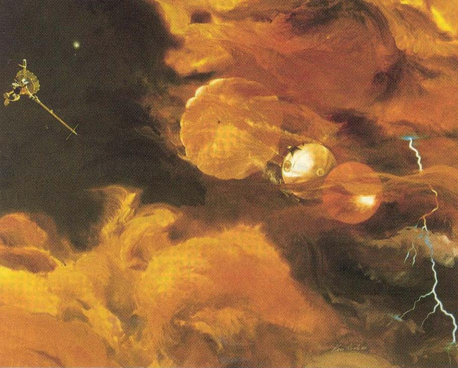
**Upon settling into orbit around Jupiter, Galileo will drop a probe into the Jovian atmosphere. As the probe descends, it will analyze samples of all of the visible cloud layers, sending its findings to the orbiter for eventual transmission to Earth. The probe is expected to transmit for about an hour and a quarter before the orbiter disappears over Jupiter's horizon.**
