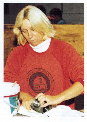
Top: Facilities maintenance mechanic **Dana Cuney gets the** old grease off with paint thinner. Eventually, rags and paintbrushes give way to a wire toothbrush to clean out all the holes and cutouts. Some of the parts have a lot of holes and cutouts. Middle: Weber uses the arbor press to seat a bearing. **Bottom: Petrie and** Weber dismantle a central gimbal assembly, a process not unlike opening a Chinese puzzle box.
