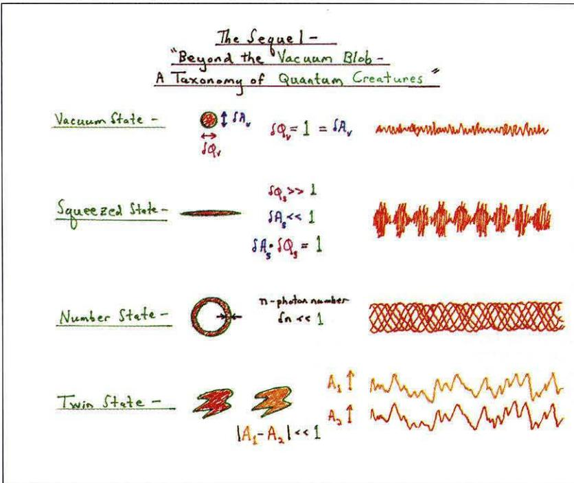
**Each column contains (from left) the name of the blob, a portrait of its fuzzball in terms of amplitude and phase, its mathematical description, and the shape of its wave. A stands for amplitude,  $\phi$  is phase, n is the number of photons, and  $\delta$  is the change or uncertainty in the variable.**
