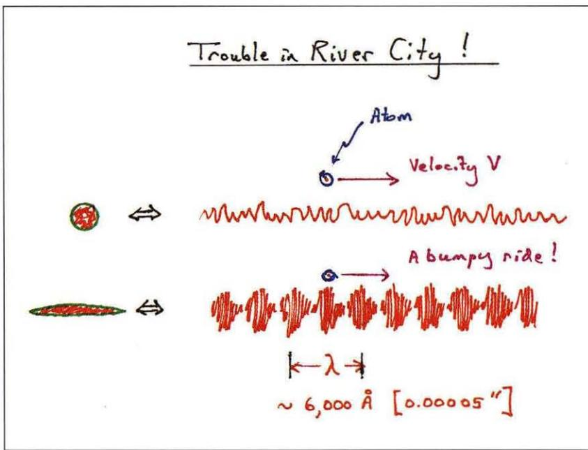
**The problem of atomic motion: An atom traveling through an ordinary vacuum (top) has smooth sailing, but an atom moving through a squeezed vacuum (bottom) is in for a bumpy ride.**
