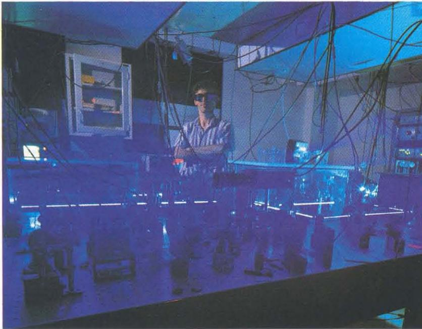
**Grad student Nikos Georgiades and the darkness-squeezing factory. The blue lasers in front of him feed into a potassium niobate crystal, where the blue photons fission into squeezed red ones. The squeezed photons emerging from the crystal are actually in the infrared region of the spectrum, and can't be seen. The dark shapes in the foreground are a part of the interferometer that they live in.**
