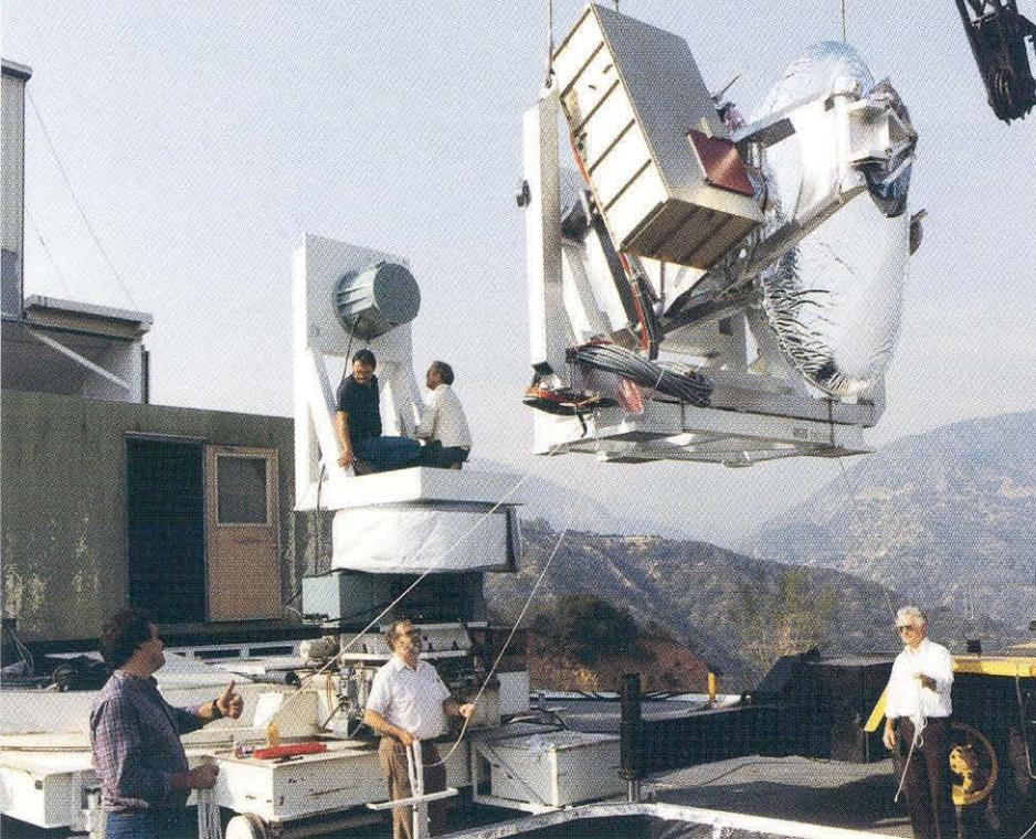
**Above:** Before being shipped east to join the rest of the spacecraft, the Microwave Limb Sounder (MLS) is mounted on the antenna range above JPL to test its reception of signal sources across the valley.
