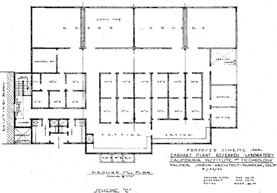
Floor plan of the projected Earhart Plant Research Laboratories at the Institute. Illustrated is the arrangement around a central hallway of four separate greenhouses and 18 light and dark rooms for controlled temperatures ranging from 2° to 30°C.
