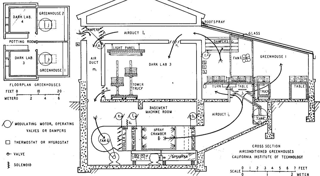
little tendency for the air to move sideways towards the exhaust slits before it had reached the ceiling. It was found essential to have the air in the plenum back up against a dead air-space before rising through the slits in the floor.
