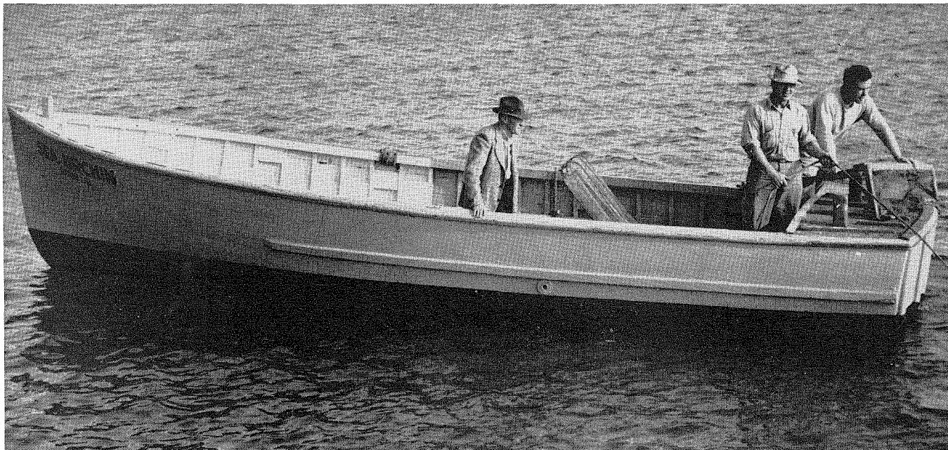
Dredging. Two dredges are shown and one is being dragged along the bottom. The dredge is towed at a rate of about 2 mph. The size of the boat is such that if the dredge fouls, the boat is held and the line does not break. A winch powered from the motor hauls up the dredge from depths of 5 to 500 ft. Deeper hauls could be made by using a bronze cable instead of rope. The dredge on the stern of the boat is the one most commonly used. Other dredges not shown are used for amphioxus and other small forms, and another type for rocky bottoms.
