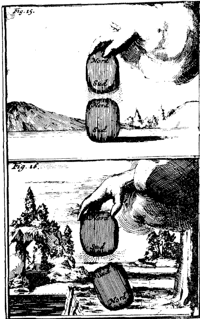
Unlike poles attract, as shown at the top, while like ones shown below repel.
