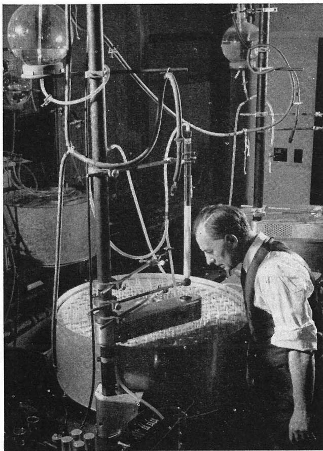
**BIOLOGY:** Electronically controlled machine built by Dr. Henry Borsook (above) and Dr. Geoffrey Keighly helps Caltech biochemists separate and collect proteins and amino acids — the fabric of all living cells.
