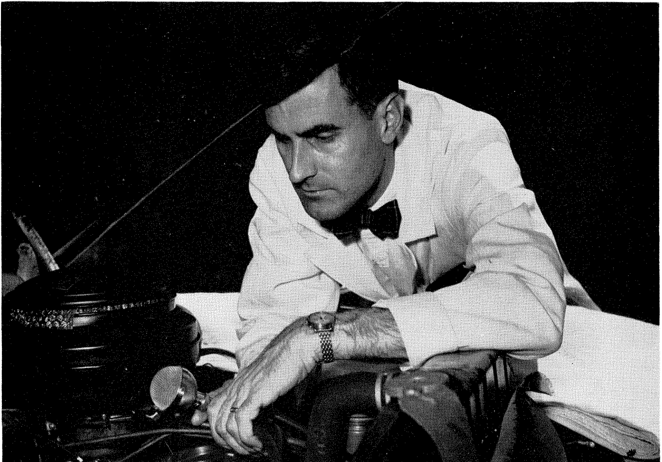
Dr. Peter Kyropoulos uses a sound-level meter microphone to measure the heart beat of an automobile engine.
