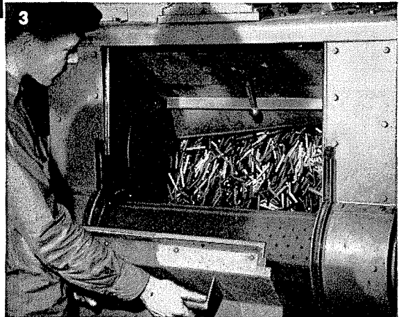
TUMBLING — Prior to inspection and packaging, REX High Speed Tool Bits are cleaned by tumbling.
