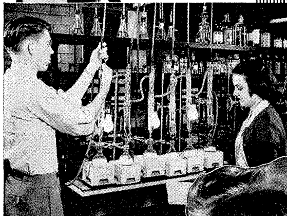
Testing action of Per-chlorethylene on various metals.
