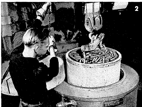
TEMPERING — Tempering is done in circulating air furnaces. All of the steps illustrated help insure a correct combination of maximum red hardness, toughness and abrasion-resistance necessary for continuous high cutting efficiency.
