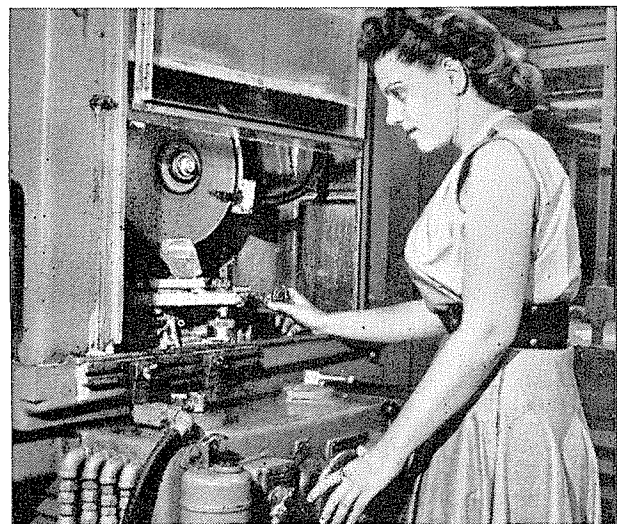
Quartz stones are cut into wafers on this diamond-edged saw, with orientation to optical axis controlled by fixture. This is just one of several types of machines designed and developed by Western Electric engineers to mechanize quartz cutting.
