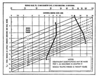
Thickness Design Charts like this (from the MS-1 manual) are used in this new computer-derived method. This chart enables the design engineer quickly to determine the over-all Asphalt pavement thickness required, based on projected traffic weight and known soil conditions.
