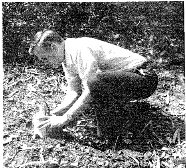
Seismometers for detecting microquakes along the San Andreas fault were originally designed to be landed on the moon to detect possible moonquakes.
