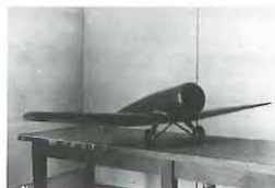
Above: Clark Millikan with a model of the DC-3 in 1935. The planes were suspended upside down for testing in the wind tunnel; the balances that weighed the aerodynamic loads are above. Right: (from left) the first aircraft tested in the tunnel, the Northrop Alpha (1930); an early version of the B-17 (1935); and the P-38 (1937).
