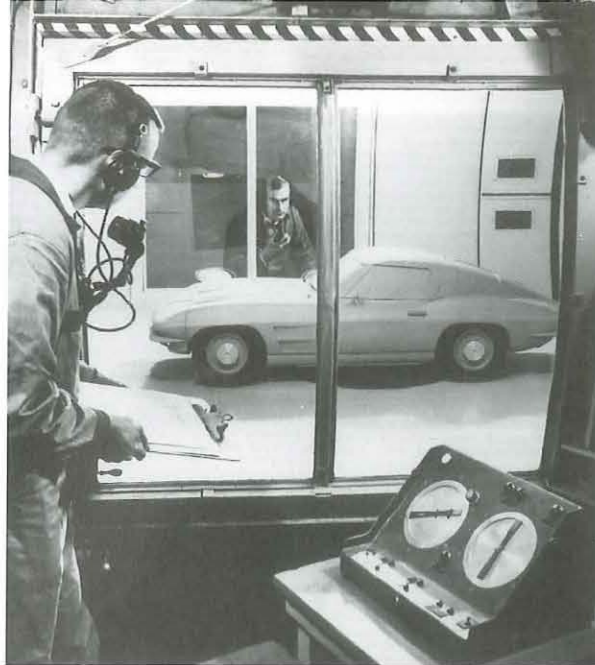
Left: The General Motors Stingray coupe was tested in the wind tunnel in 1959 (it came on the market in 1963).
