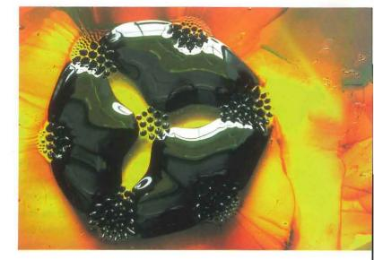
A drop of ferrofluid (part liquid, part magnet) on glass flows into a unique shape determined by magnets placed underneath. Photo by Felice Frankel in On the Surface of Things.
