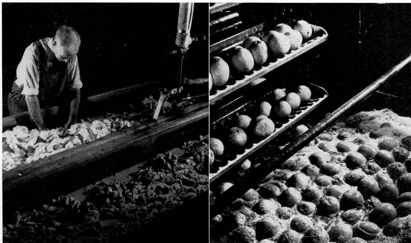
FIG. 5. AT LEFT: Soap has a role in many industrial processes. Here raw silk for parachutes and shroud lines gets a "soaking" bath as an important step in its processing. FIG. 6. AT RIGHT: First step in the packing house in preparing oranges for market is the soap-and-water bath. On the left, a carrier removes oranges from the suds and takes them up to be rinsed with warm and cold showers, then dried by brushes and warm air currents.
