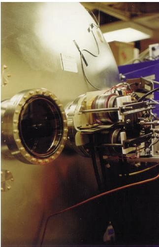
**Above: The plasma gun is mounted on one end of the vacuum chamber, next to a viewport. The stubby cylinders are magnetic coils that generate a magnetic field of 3 kilogauss—typical of sunspots, with which active prominences are normally associated, and 10,000 times stronger than Earth’s surface field at the equator. The electric field that twists up the prominence is created by a 200-pound capacitor that can deliver 72,000 amps in five millionths of a second.**
