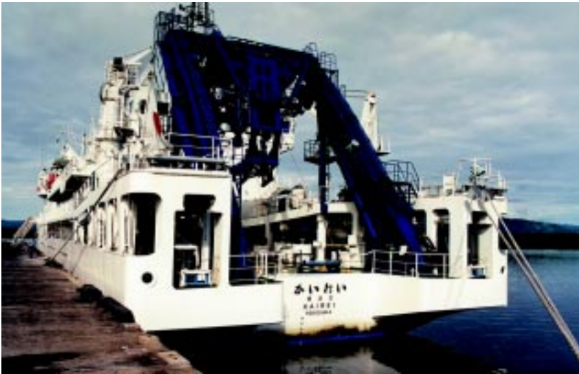
Above: Launched in 1997, the RV Kairei is designed to stay at sea for months at a time. She's 105 meters long overall, displaces 4,628 gross tons, and has a crew of 29—not counting up to 31 scientists. The big blue thing is an A-frame designed to lower corers, sonar arrays, or even robot submarines. Below, left: Pirates are a big problem in the South Pacific, so the Kairei sported a barbed-wire girdle when not in port. Fire hoses and stacks of bamboo staves were kept ready at all times to repel boarders. Below: These guys weren't exactly pirates, but they may have been smugglers—they approached the ship expectantly, says Watts, but eventually left when nothing was thrown overboard for them to retrieve. Whatever they were, they were bold seafarers—the Kairei was roughly 100 kilometers from the nearest land at the time.
