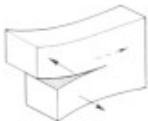
Mode III cracks tear a material by shearing it perpendicularly to their direction of travel.
