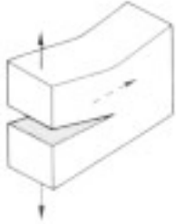
Mode I cracks open a material perpendicularly to their direction of travel.
