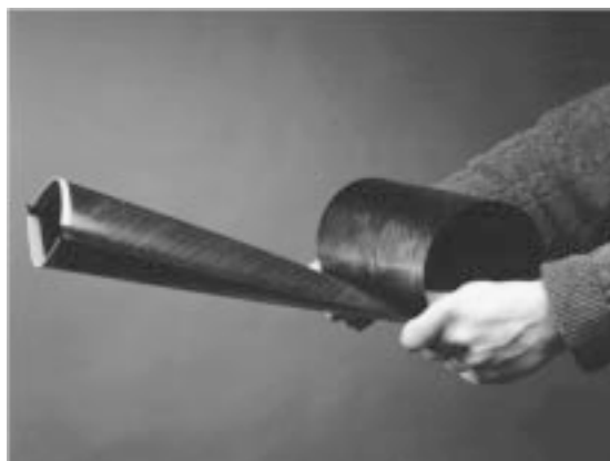
Above: The Carnegie-Mellon heliogyro. Right: The DLR's lens-shaped boom will be used in ESA's solar-sail program, which is planning a test flight in a year or so.
