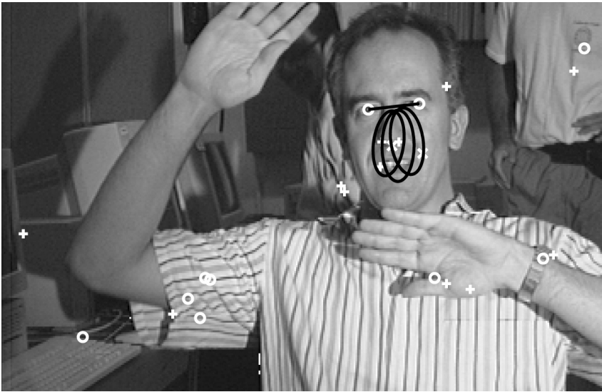
Above: In this shot of Perona's face, the circles mark all the features the computer thinks could be eyes, the + 's are nostrils, and the X 's are nose tips. The computer picks a pair of eye candidates (the correct one, as it happens), and searches the central ellipse for a nose tip and the side ellipses for nostrils.
